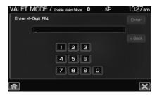
**Note:** The PIN can be reset by simultaneously pressing and holding presets 1 and 5 while on the PIN entry screen. After approximately five seconds, the system will transition to the Valet mode screen indicating that the PIN is reset. Once you have reset the PIN, the system will then allow you to set a new PIN.
